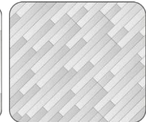
3-board stagger diagonal
